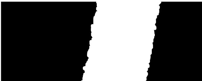
6. Least-squares fit each edge to a line, and rotate image by angle between the hair and vertical.
