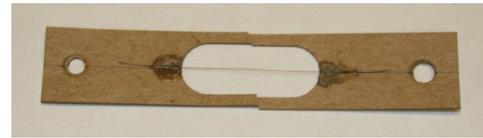
Fig. 4. Test grip used to hold the hair. The hair is glued to rigid fiberboard to prevent stress concentrations from forming from mechanical clamping on the hair itself.
